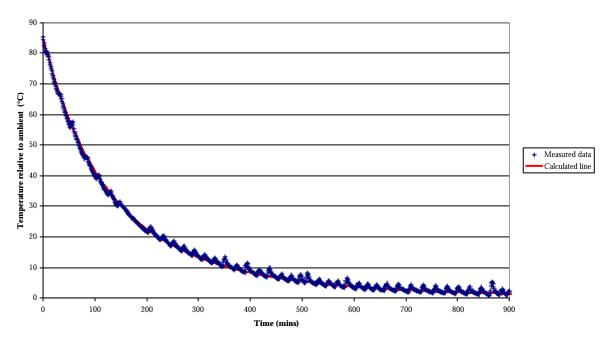
Heating curve for VW Golf TDi at 0°C ambient with corrected time
