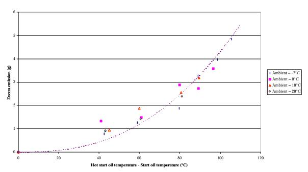
Figure 3 shows an example of the comparison between excess CO emissions calculated from the empirical equations and the experimentally measured values for a range of vehicles, conducted under the reduced test matrix with a range of ambient and starting temperatures. The agreement is very good which shows that the empirical equations represent the actually measured data very well.
