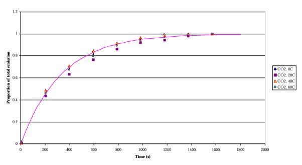
Proportion of total CO<sub>2</sub> emissions as a function of time into cycle at an ambient temperature of 0°C for VW Golf
