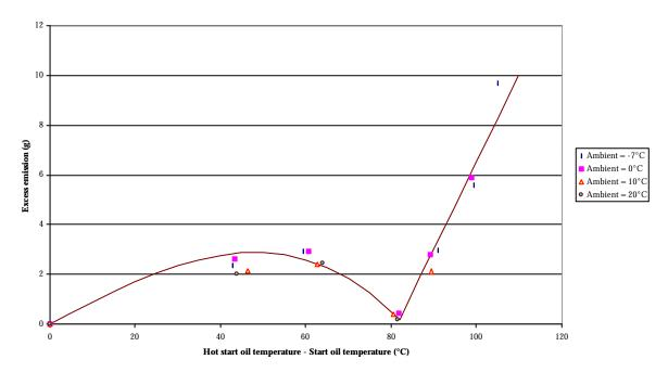
Although the form of this curve can be very different dependent on the vehicle and pollutant, the same basic independence of ambient temperature was found. For example, Figure 2 shows the curve for CO excess emissions from the diesel-fuelled VW Golf.
