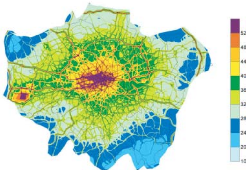
Figure 6.56 Annual mean NO 2 concentrations for 2001 in London estimated using the ERG model ( \mu\text{g m}^{-3} ).
