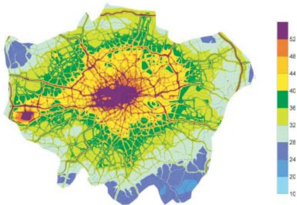
Figure 6.55 Annual mean NO 2 concentrations for 1999 in London estimated using the ERG model ( \mu\text{g m}^{-3} ).
