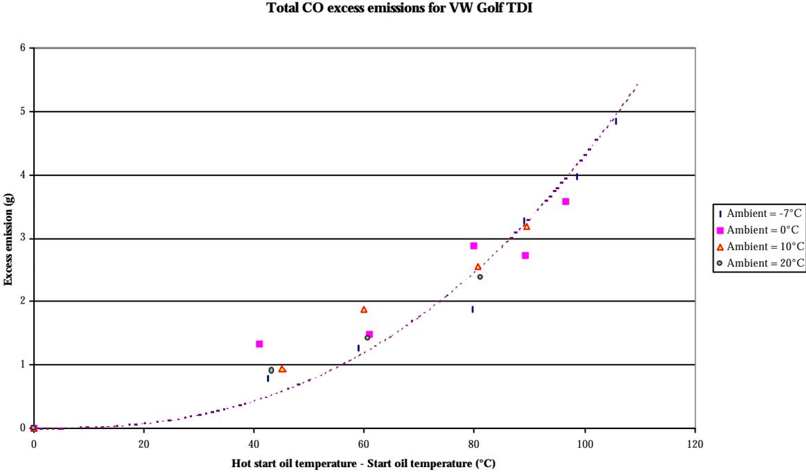
Figure 3 shows an example of the comparison between excess CO emissions calculated from the empirical equations and the experimentally measured values for a range of vehicles, conducted under the reduced test matrix with a range of ambient and starting temperatures. The agreement is very good which shows that the empirical equations represent the actually measured data very well.
