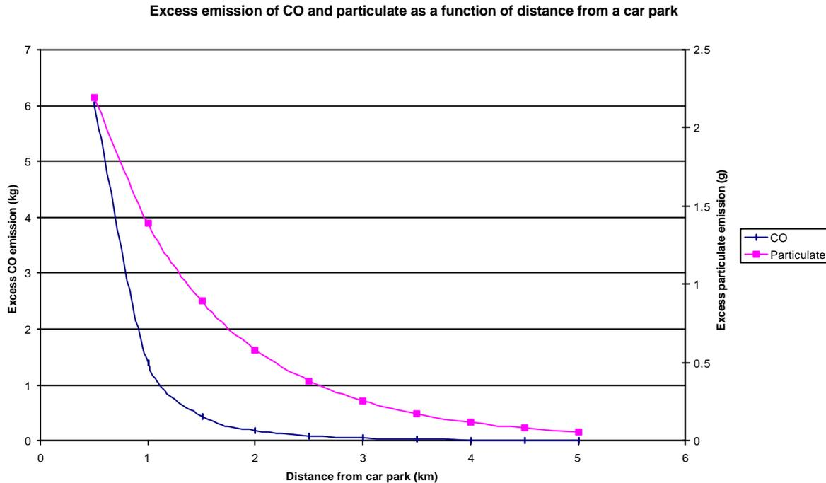
The model can simulate many different car parking arrangements. For example, the parking time might be different if the car park is for a shopping centre (a distribution of parking times could be used). The vehicles may not arrive in a hot condition so that the excess leading to the car park has to be included in the calculation. The vehicles may not all drive beyond 5km from the car park, etc. The change with time of day could be simulated with changes in vehicle number and ambient temperature.
