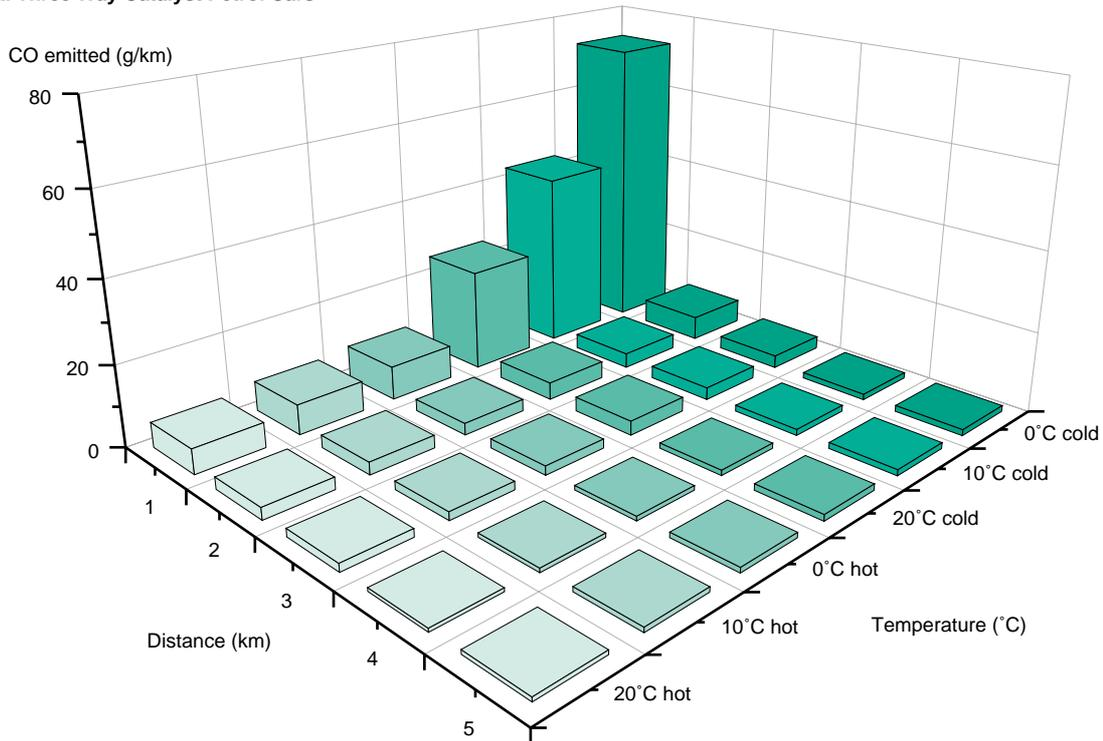
Note: Average emissions from 6 TWC cars tested over a TRL driving cycle designed to simulate the "commute to work" journey.
