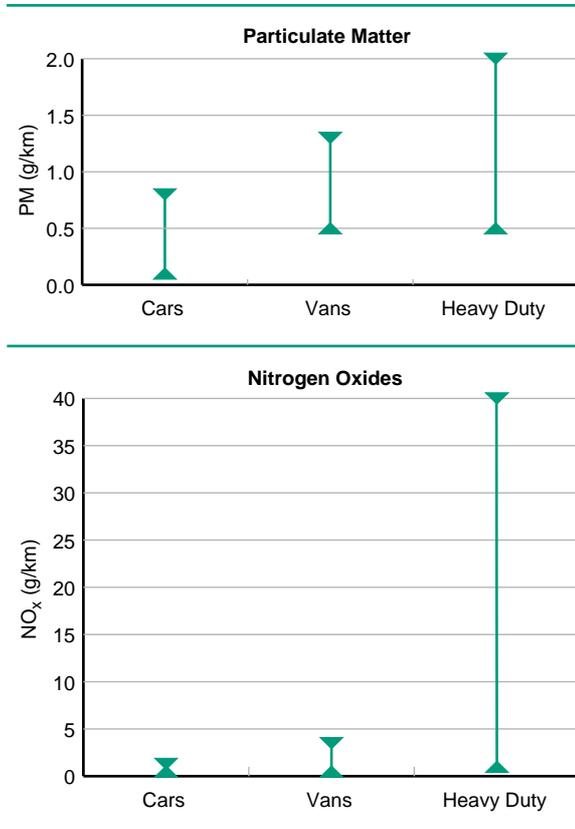
Note: The large range of emissions for heavy duty vehicles reflects the wide range of vehicle types, sizes and technology in this category and the effect of laden weight on emissions, particularly of NO<sub>x</sub>.
