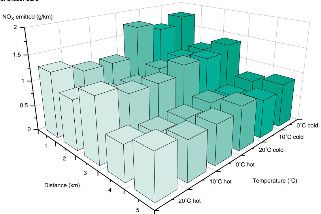
Note: Average emissions from 3 diesel cars tested over a TRL driving cycle designed to simulate the "commute to work" journey.
