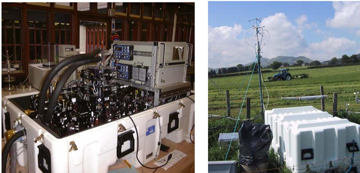
**Figure 5.5.** Dual-channel  $\text{NH}_3/\text{HNO}_3$  lead salt tunable diode laser tested for eddy-covariance measurements at Easter Bush.
