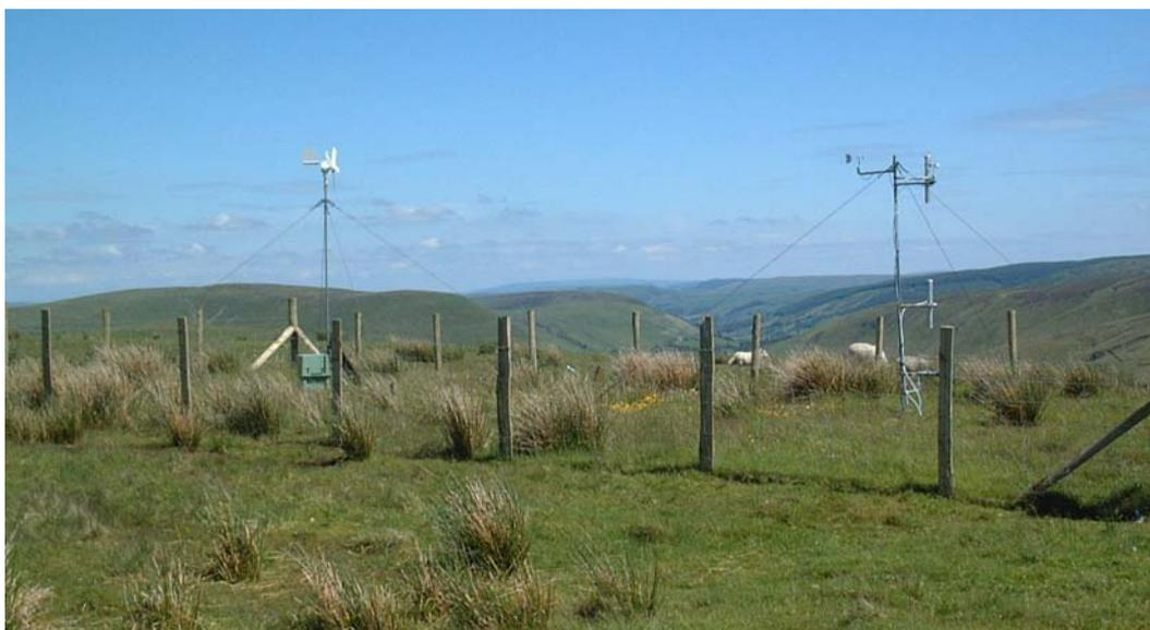
**Figure 5.7.** Time Averaged Gradient (TAG) system for  $\text{NH}_3$  at Plynlimon (right mast), powered by wind and solar power (left mast).
