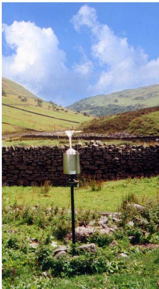
Figure 4 Bulk rain sampler (Bannisdale)
