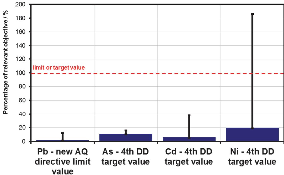
**Figure 4.** A summary of the annual mean measured concentrations of the heavy metals relevant to the New Air Quality Directive and Fourth Daughter Directives on the UK Heavy Metals Monitoring Network in 2013 as a percentage of the relevant air quality objectives. The bars indicate the annual mean of all sites; the lines indicate the annual mean at the site with the highest concentrations.
