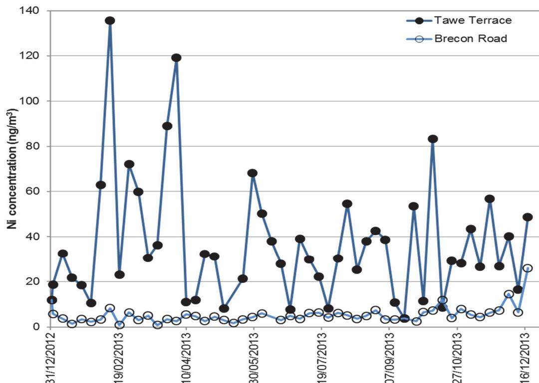
**Figure 9.** Measured Ni concentrations at Site 113: Pontardawe Tawe Terrace and Site 115: Pontardawe Brecon Road, in 2013 (both sampled weekly).
