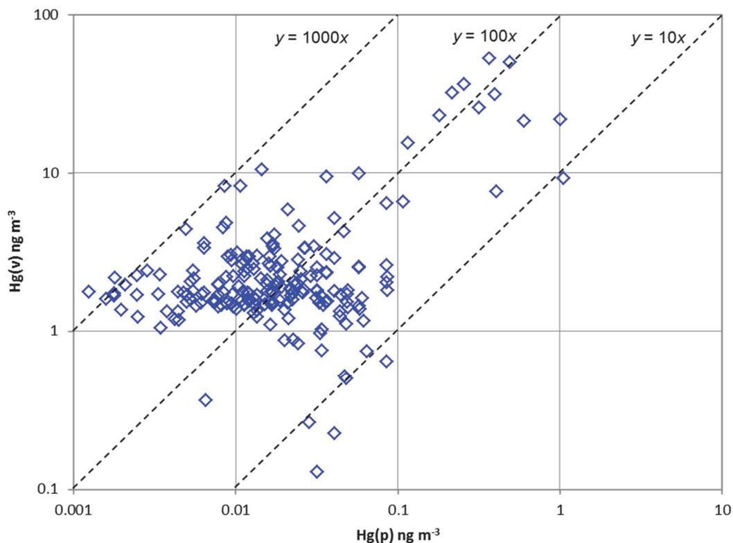
**Figure 11.** The relationship between monthly particulate [Hg(p)] and total gaseous [Hg(v)] mercury measurements during 2013 where these are made together. The dotted diagonal lines represent the locus of points for which the total gaseous mercury concentration ( $y$ ) are 10, 100 and 1000 times greater than the measured particulate phase mercury concentrations ( $x$ ), as indicated.
