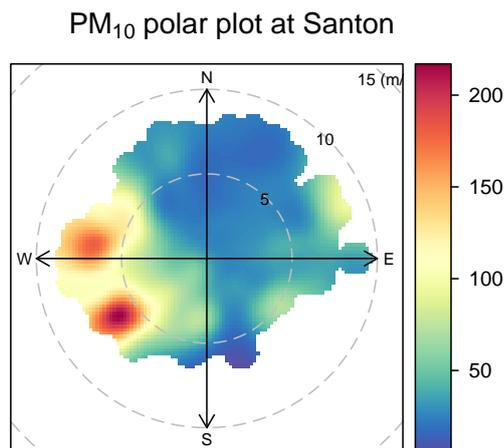
**Figure 1:** Polar plot showing concentrations of PM<sub>10</sub> at Santon, as a function of wind speed and direction.
