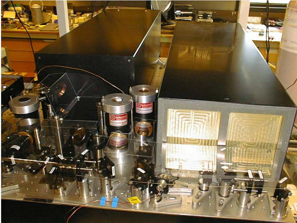
**Figure 2.3** A photograph of the lidar showing the laser enclosure, the optical mounts, the detectors and the telescope.
