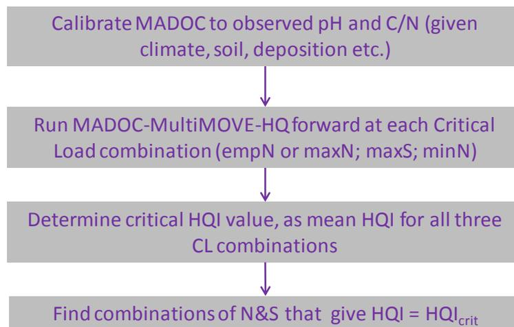
**Figure 4.** Workflow for using the MADOC-MultiMOVE model chain to derive a biodiversity-based critical load function describing combinations of nitrogen (N) and sulphur (S) pollution above which a habitat quality index (HQI) is reduced to below a critical level.
