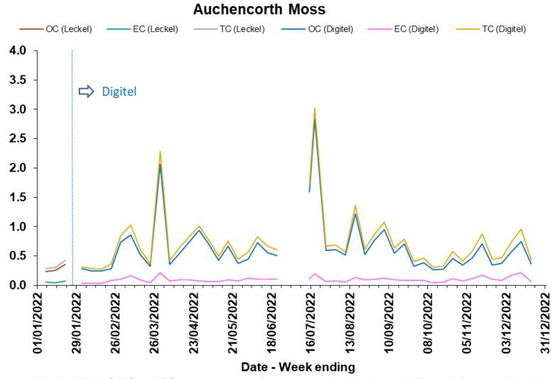
Figure 34 - Weekly PM<sub>2.5</sub> OC, EC, and TC mass concentrations measured at Auchencorth Moss during 2022. Note that the data from 9-20 July are plotted as weekly averages calculated from daily samples. All other data are from weekly samples
