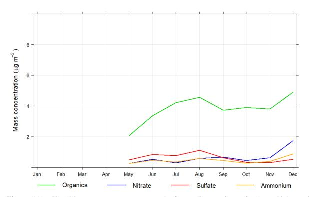
Figure 22 - Monthly average mass concentrations of organics, nitrate, sulfate and ammonium in  $PM_1$  measured by ACSM in 2022 at London Marylebone Road
