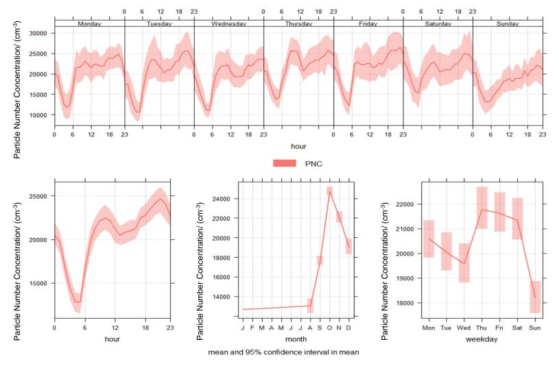
Figure 12 - Temporal variations of particle number concentrations in 2022 at London Marylebone Road. Note that any line joining non-consecutive months in the monthly plot is automatically produced by the software used to generate the plot and is not intended to represent the particle number concentration of the 'missing' month(s).
