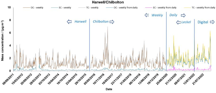
Figure 35 - Time series of the weekly OC, EC, and TC mass concentrations in the  $PM_{2.5}$  fraction at Harwell/Chilbolton Observatory since the installation of the sampler up to June 2020 and daily mass concentrations from 11 June 2020. The sampler was replaced by a Digitel sampler in January 2022. The daily mass concentrations measured since June 2020 have been plotted as calculated weekly average for consistency.
