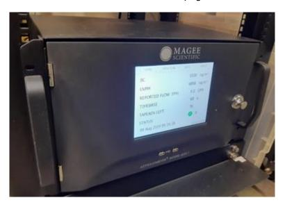
Figure 9 - Aerosol Magee Scientific AE33 Aethalometer, photograph courtesy of NPL.
