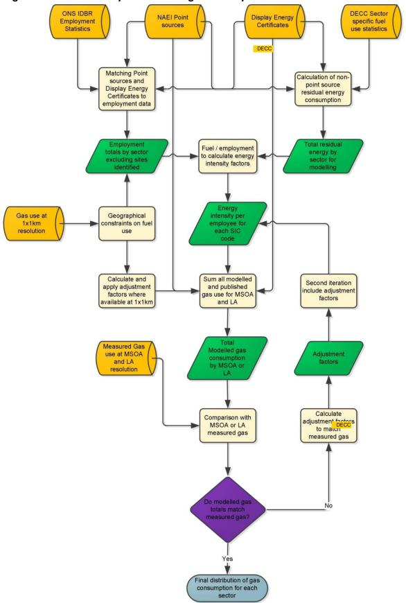
Figure 3.3: Gas consumption modelling data and process flow
