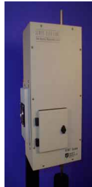
FDMS Main Enclosure.
