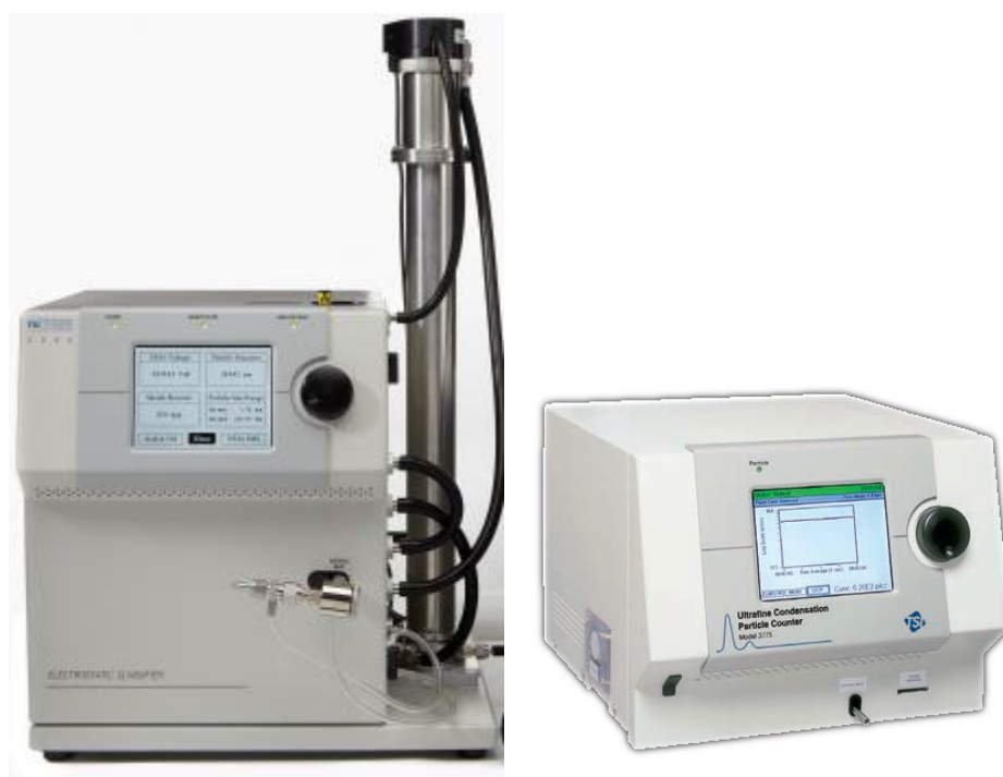
Figure 1 - SMPS TSI 3936L75, consisting of an electrostatic classifier TSI 3080 and a long differential mobility analyser TSI 3081 (left), and condensation particle counter TSI 3775 (right).
