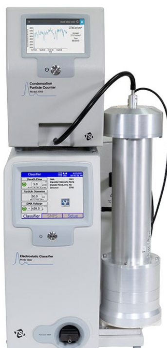
Figure 2 - SMPS TSI 3938W50-CEN-7, consisting of an electrostatic classifier TSI 3082 and a wide-range differential mobility analyser TSI 3083 (bottom), and condensation particle counter TSI 3750-CEN-7 (top).
