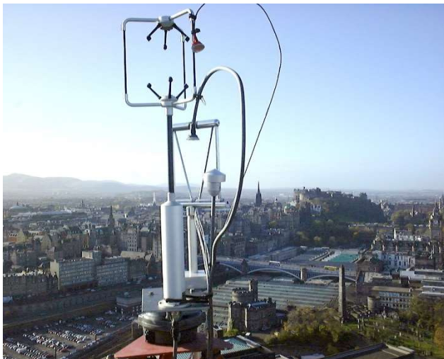
Figure 4.2 Eddy-covariance instrument and inlet above the city of Edinburgh consisting of an ultrasonic anemometer, a fast-response hygrometer and several inlets leading to fast-response particle analysers.
