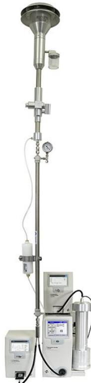
**Figure 4 - (left to right) TSI 3750-CEN-7 CPC; TSI 3750200 sampling/drying system; and TSI 3938W50-CEN-7 SMPS, consisting of TSI 3082 electrostatic classifier, TSI 3083 DMA, and TSI 3750-CEN-7 CPC. Photograph courtesy of TSI Incorporated.**
