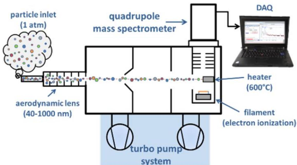
Figure 5 - ARI Q-ACSM schematic diagram (DAQ = Data acquisition [control]). Image copyright of Deutscher Wetterdienst (DWD).
