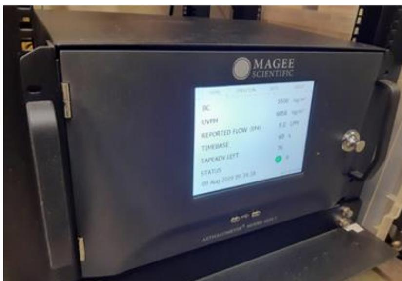
**Figure 9 - Aerosol Magee Scientific AE33 Aethalometer, photograph courtesy of NPL.**
