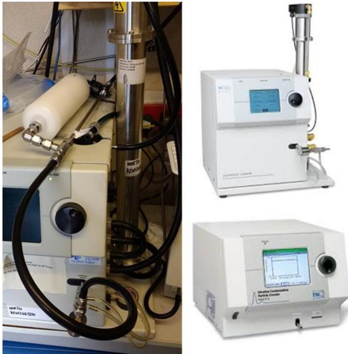
**Figure 3 - NPL drying unit, (left); TSI 3936 SMPS, consisting of: TSI 3080 electrostatic classifier and TSI 3081 DMA (top-right); and TSI 3775 CPC (bottom-right). Photographs courtesy of NPL, Envco, and TSI Incorporated respectively.**
