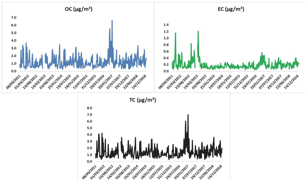
**Figure 4-4 Time series of OC, EC and TC in the PM<sub>2.5</sub> fraction at Harwell/Chilbolton since the installation of the sampler up to the end of 2018 (weekly samples) (µg/m<sup>3</sup>). The sampler moved from Harwell to Chilbolton in February 2016.**
