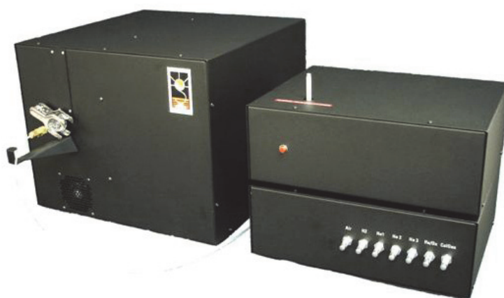
Figure 2-4 Sunset Laboratory Inc. thermal/optical carbon analyser
