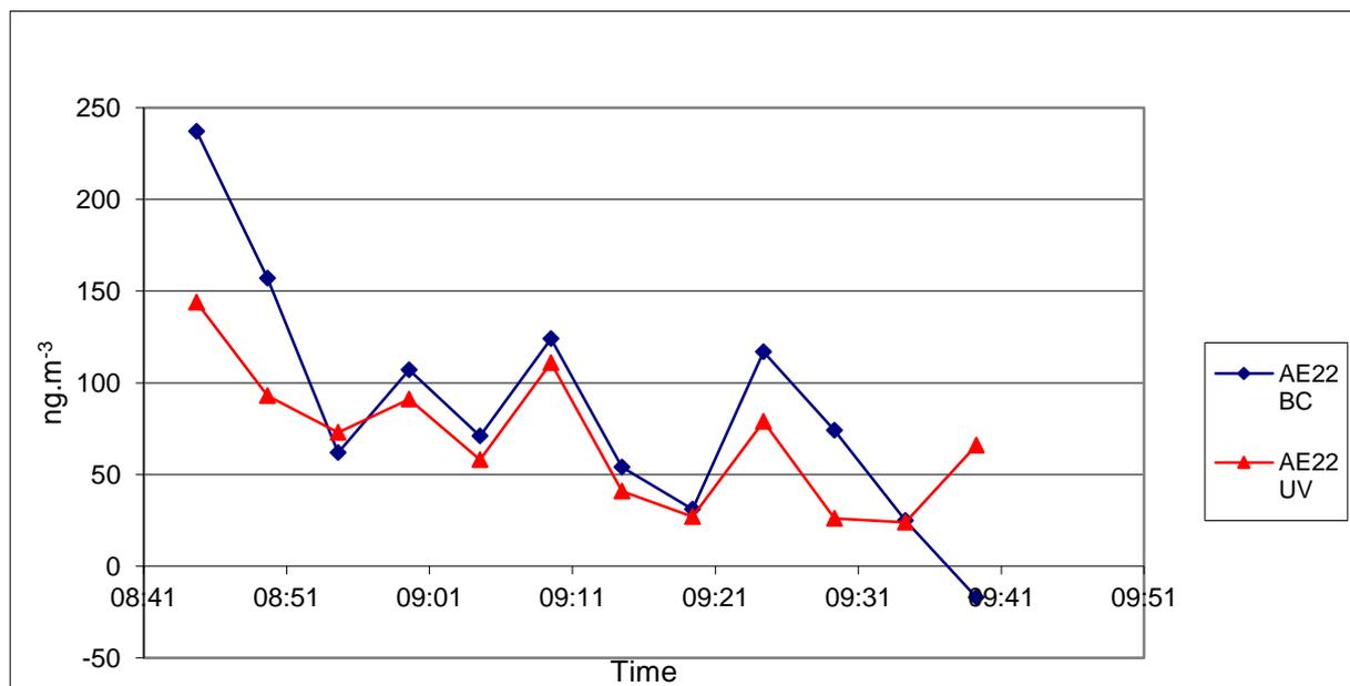
**Figure 3 Strabane Aethalometer sampling HEPA filtered air**
