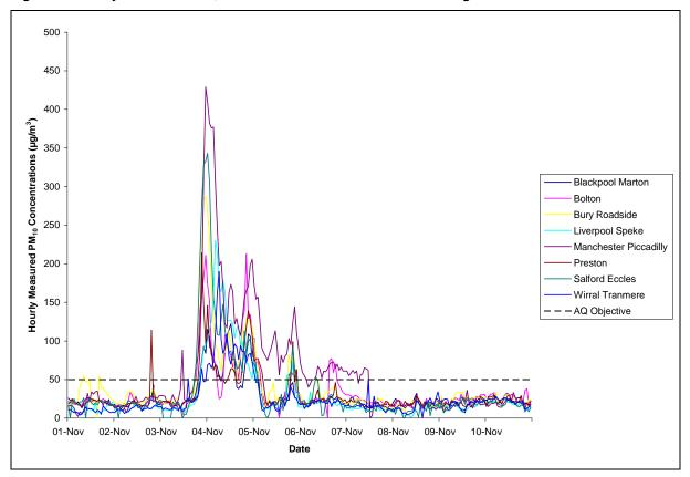
Figure 1.2 Hourly Measured PM<sub>10</sub> Concentration in the North East of England
