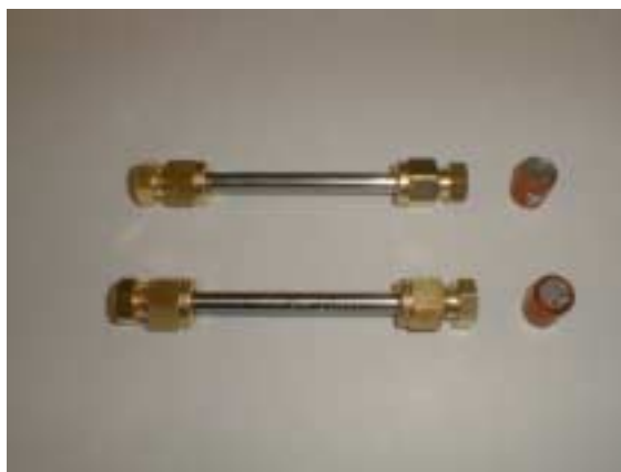
Figure 2.2(a): Capped benzene and 1,3-butadiene diffusion tubes
