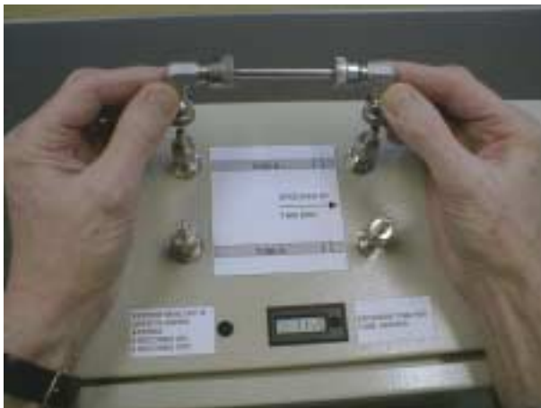
Fig 2.10(a) Installation of a new tube
