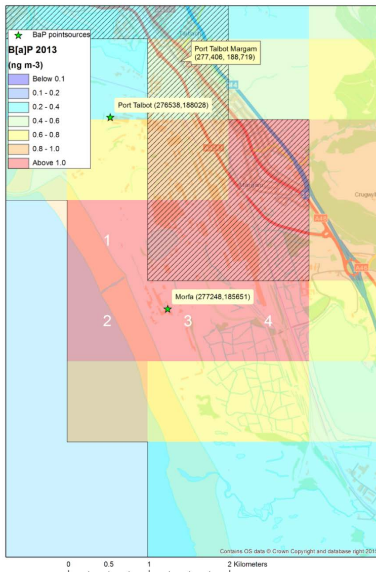
Figure 2 Exceedance situation South Wales [B[a]P_UK0041_2013_1]. Exceeding grid squares are marked red. Locations of coke works at Morfa and sinter plant at Port Talbot are also shown. Non-hatched grid squares are those assigned to South Wales zone UK0041. Hatched grid squares are assigned to Swansea Urban Area zone UK0027 and do not form part of this exceedance situation.
