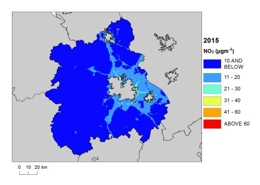
Figure 5: Map of modelled roadside annual mean  $NO_2$  concentrations 2015. Modelled exceedances of the annual limit value are shown in orange and red.
