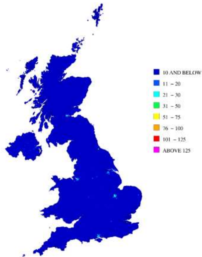
Figure 5-2 99.18 th Percentile of 24-hour Mean SO 2 Concentration, 2017 ( \mu\text{g m}^{-3} )
