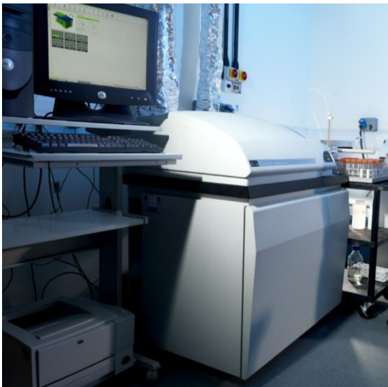
Image 2: One of two dedicated ICP-MS instruments comprising the UK ambient metals analysis facility at NPL.
