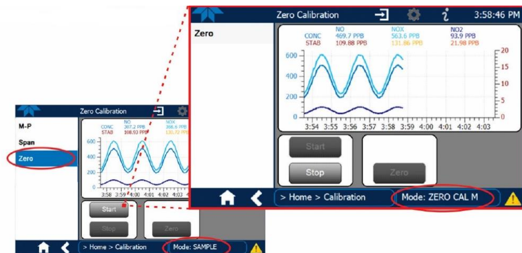
Figure 10 - Starting zero calibration with a scrubber on API T200 with NumaView. ©Teledyne API
