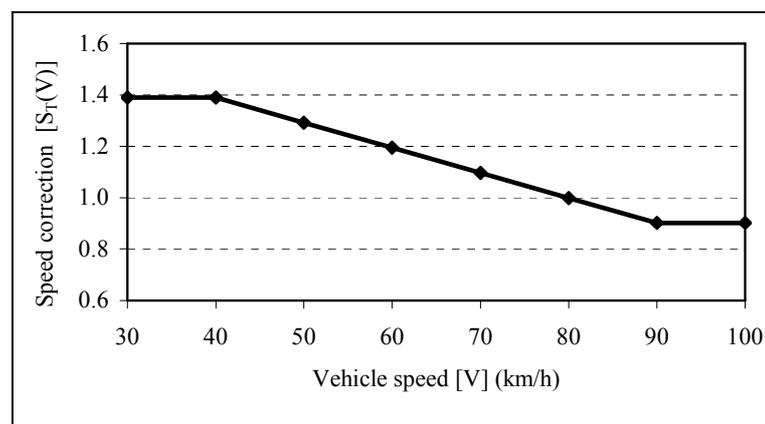
Figure B1: Speed correction factor( $S_{T(V)}$ ) for tyre wear particle emissions.
