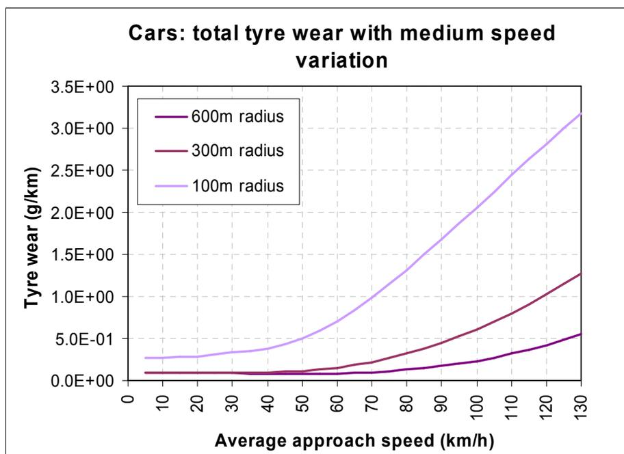
Figure 8: Car tyre wear as a function of average road curvature based on mechanistic model proposed for HDM-4.
