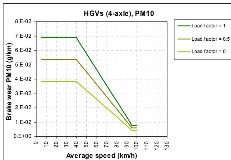
Figure 6: PM<sub>10</sub> emission factors for brake wear on 4-axle HDVs as a function of vehicle load.
