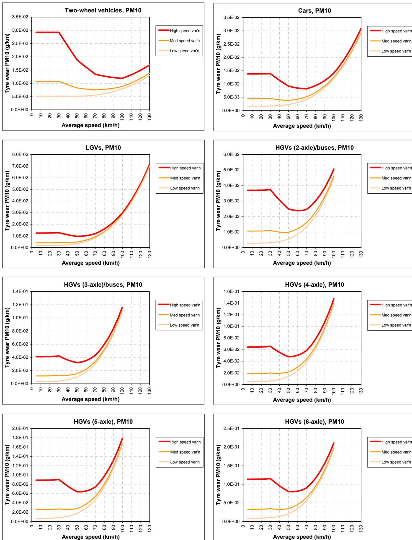
Figure 9: PM<sub>10</sub> emissions for different vehicle categories, based on HDM-4 tyre consumption model for a road radius of 573m and three levels of speed variation.
