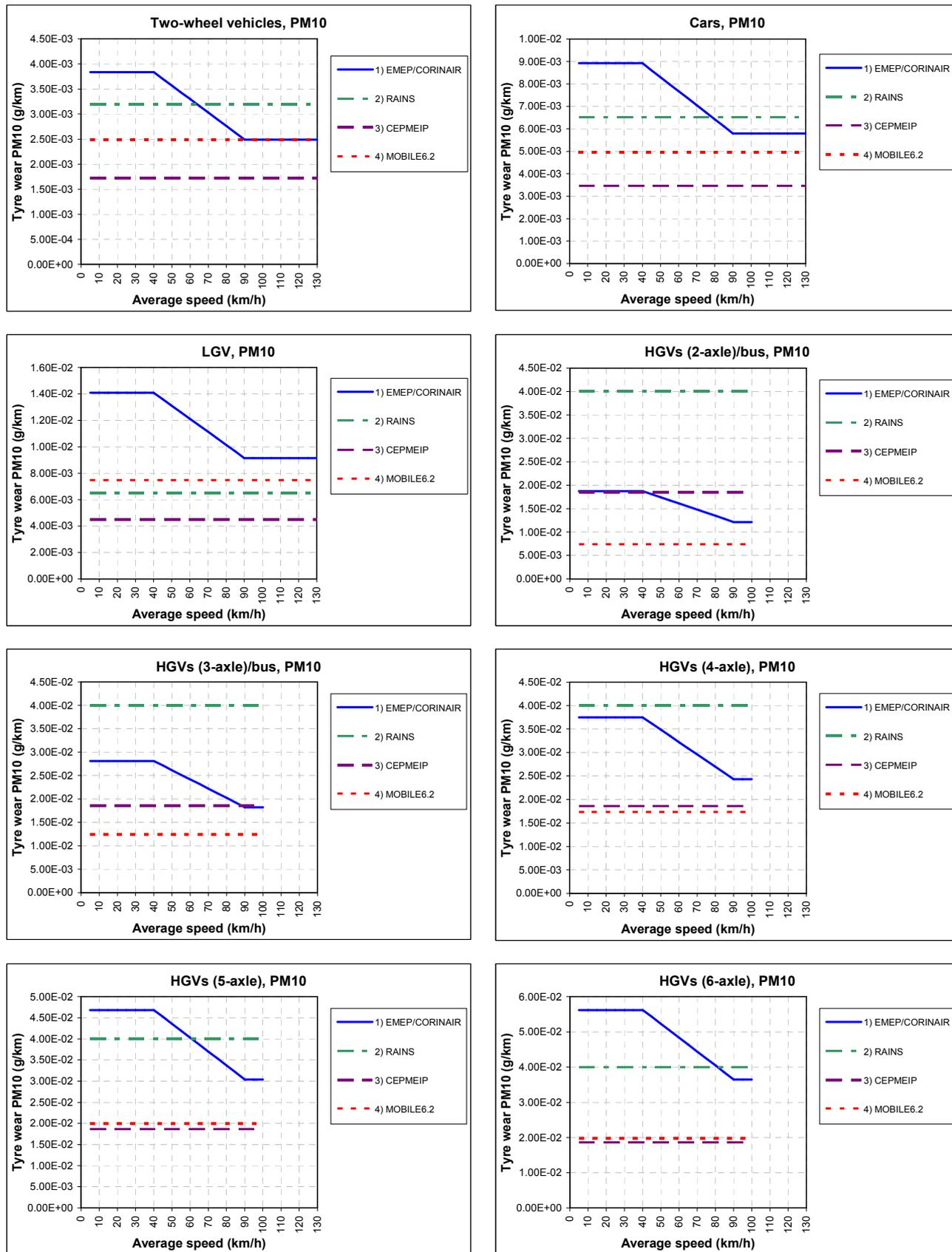
Figure 1: PM<sub>10</sub> emission factors for tyre wear by vehicle type and emission model.
