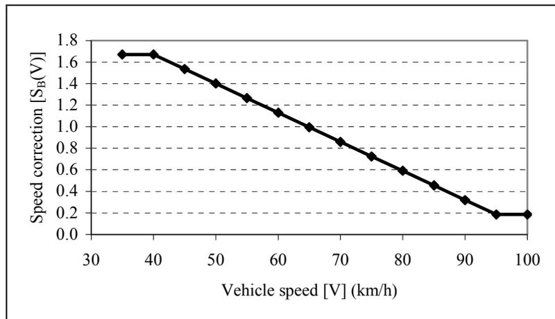
Figure E2: Speed correction factor ( $S_{B(V)}$ ) for brake wear particle emissions.
