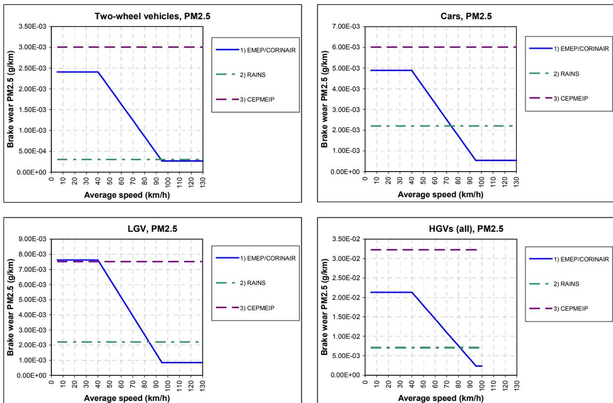
Figure 5: PM<sub>2.5</sub> emission factors for brake wear by vehicle type and emission model.
