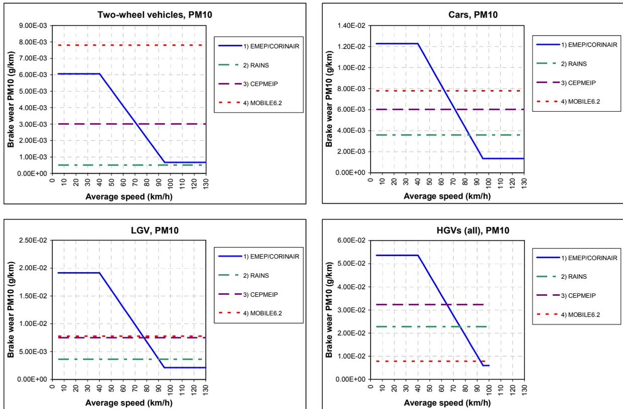
Figure 4: PM<sub>10</sub> emission factors for brake wear by vehicle type and emission model.
