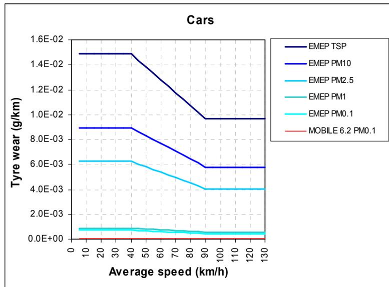
Figure 3: PM emission factors for car tyre wear by size fraction.
