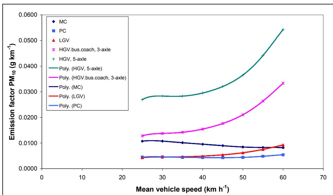
Figure 24: Relationships between mean vehicle speed and tyre wear PM<sub>10</sub> emission factors for the main vehicle categories (medium speed variation and 435 m road radius).
