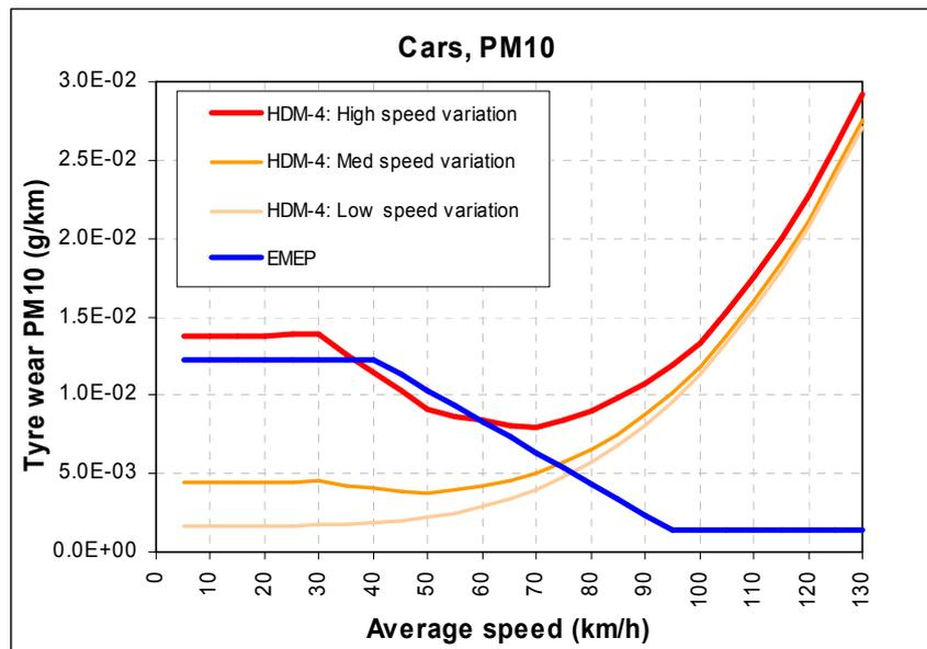
Figure 10: Emissions of PM<sub>10</sub> due to car tyre wear predicted using the EMEP method and a method based upon the mechanistic tyre consumption model in HDM-4 (for an average road radius of 600 m and three levels of speed variation).
