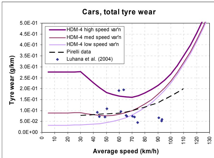
Figure 7: Tyre wear predictions based on mechanistic model proposed for HDM-4 (road radius = 573m). Data from the PARTICULATES project (Luhana *et al.*, 2004) and Pirelli are shown for comparison.
