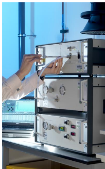
Image 2: (Far left) One of two dedicated ICP-MS instruments comprising the UK ambient metals analysis facility at NPL.
