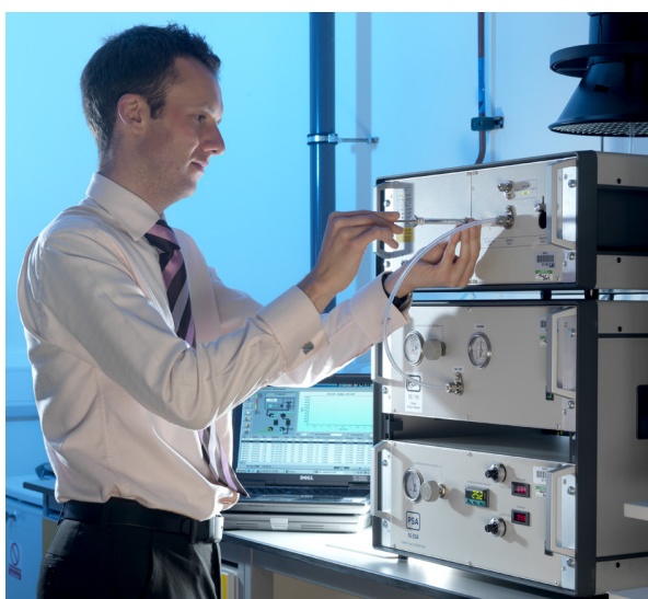
Image 4: One of two thermal desorption-atomic fluorescence analysers comprising the UK total gaseous mercury analysis facility at NPL.
