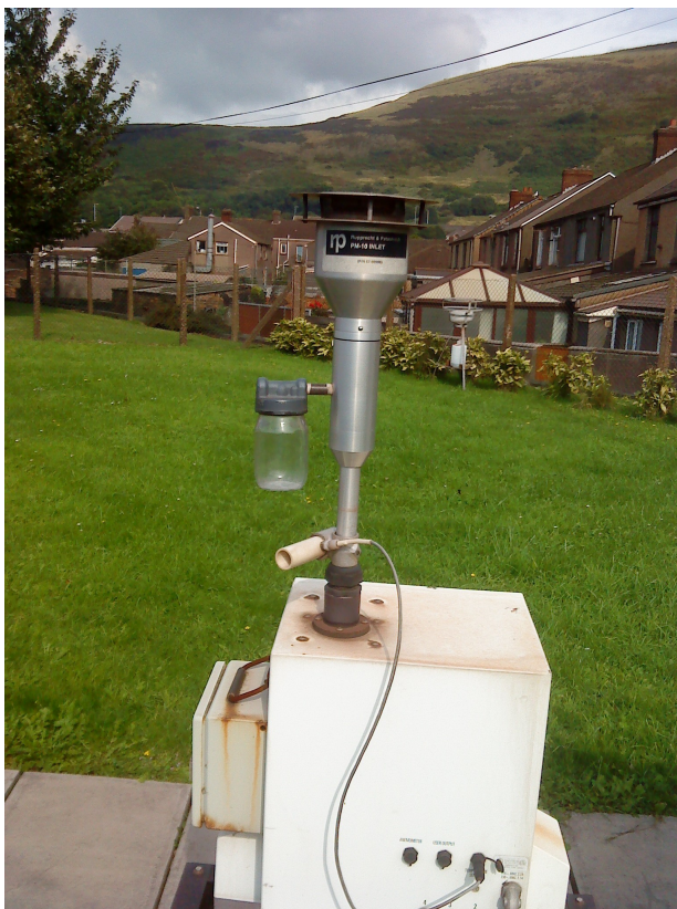
Image 1. The Partisol 2000 sampler at the Port Talbot Margam Network site prior to its 2010 annual audit.
