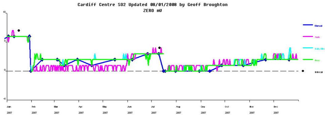
**Figure 8.1. Calibration Control Charts for SO<sub>2</sub> Analyser Zero Baseline.**
