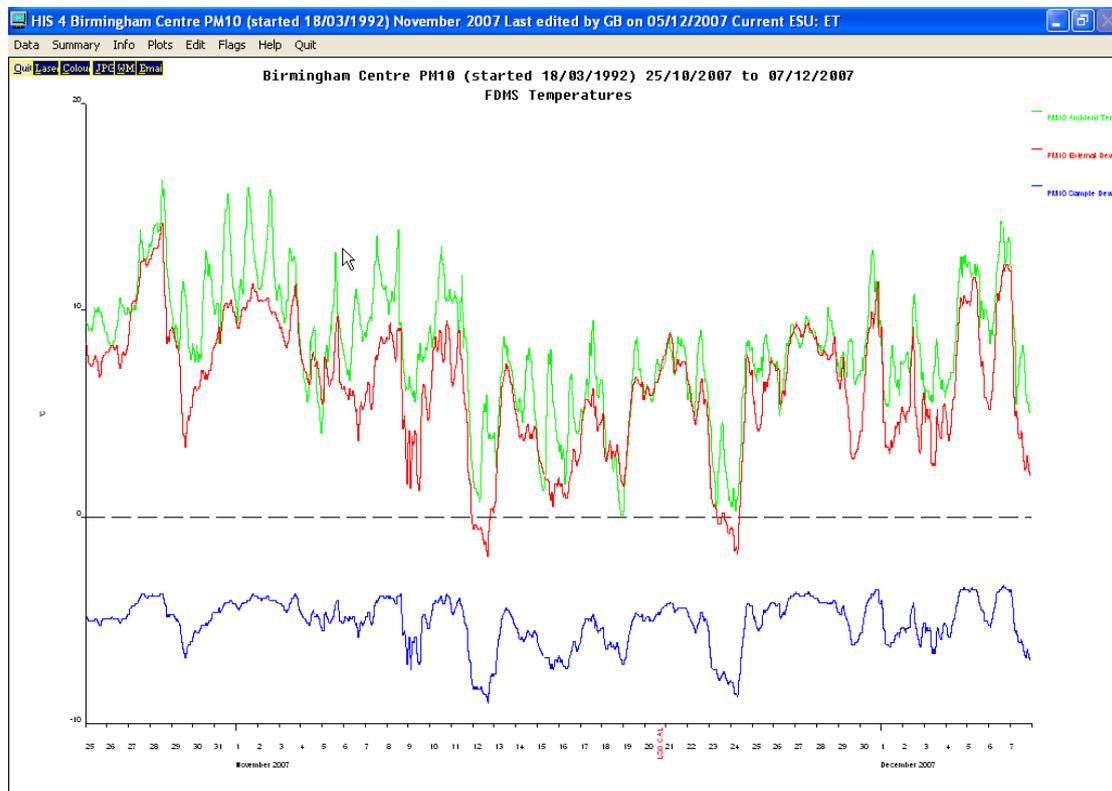
**Figure 8.7. Temperature Time-series for an FDMS instrument**
