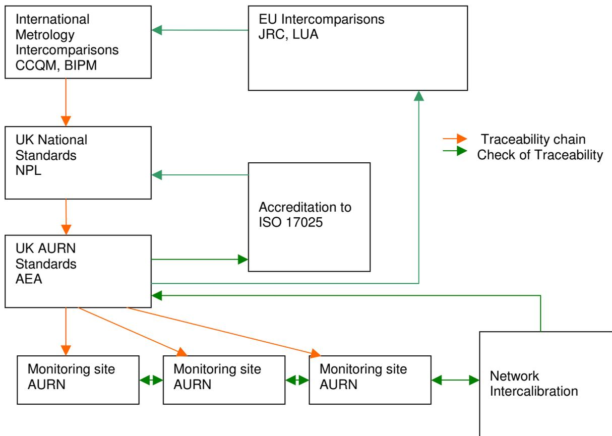
Figure 9.1 Traceability chain and traceability checks for UK AURN gaseous measurements
