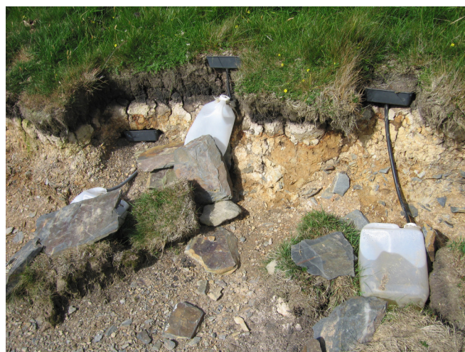
Figure 3.9b: Tray lysimeters at Afon Gwy showing different horizons sampled
