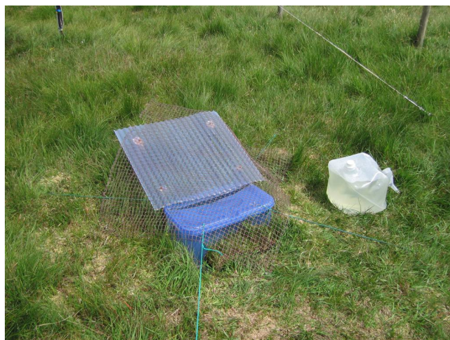
Figure 3.9a: High volume bulk deposition collector at Afon Gwy flume
