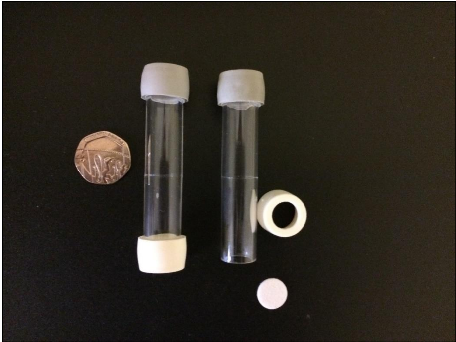
Figure A.1: Diffusion Tube with Wind-Protection Cap
