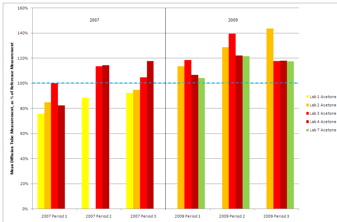
Figure 3-9 Comparison of percentage bias of 50% TEA/acetone diffusion tubes in 2007 and 2009 3-month field studies (each bar is mean of 6 replicates)
