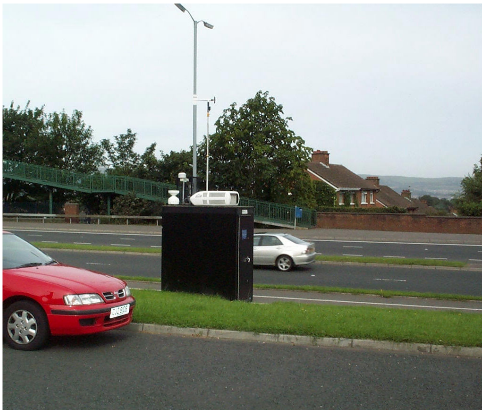
Figure 4.2 New monitoring site for NO x (and PM 10 ), Loughview Drive, Castlereagh
