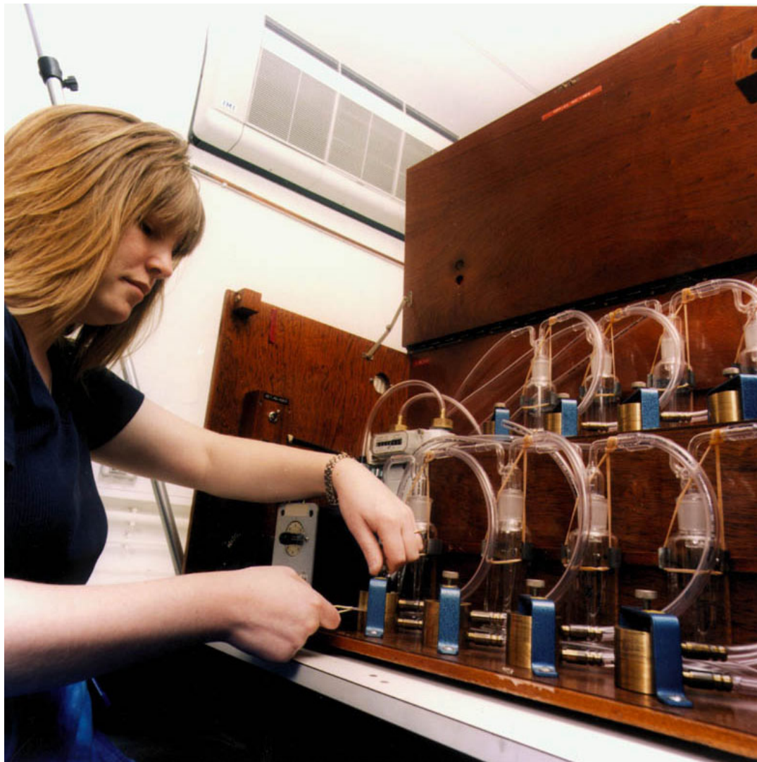
Figure 5.3 8-port Sampler for Smoke and SO 2
