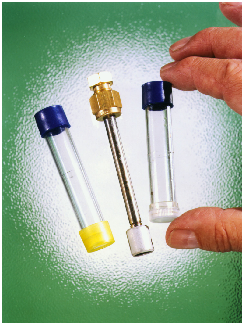
Figure 4.3 A Selection of Diffusion Tubes (from left to right, SO 2 , BTX, NO 2 )
