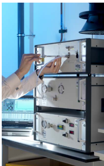
Image 3: (Far left) One of two dedicated ICP-MS instruments comprising the UK ambient metals analysis facility at NPL.
