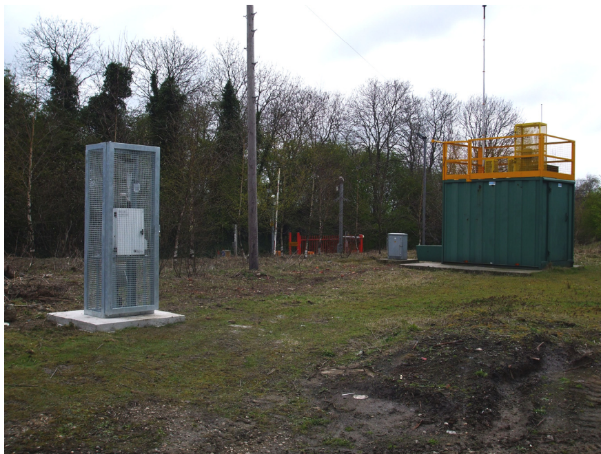
Image 2. The renamed Network monitoring site at Scunthorpe Low Santon. The Network sampler is in the grey cage on the left of the picture.
