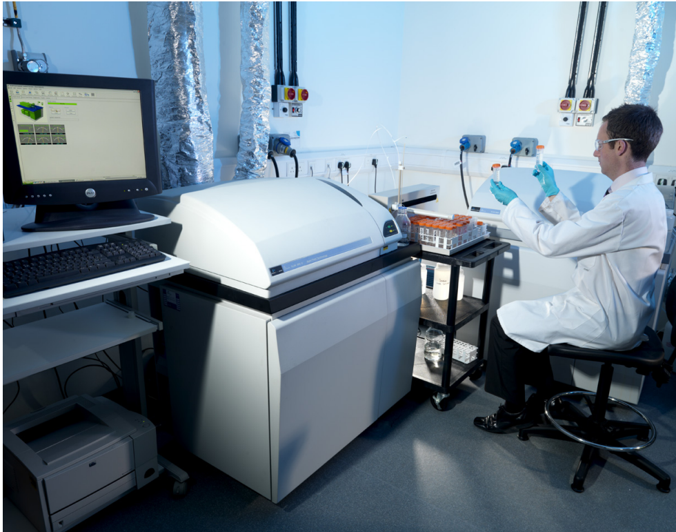
Image 5: One of two dedicated ICP-MS instruments comprising the UK ambient metals analysis facility at NPL.
