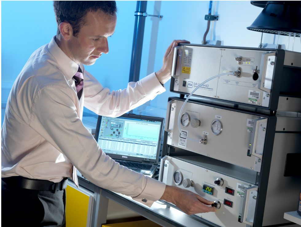
Image 6: One of two thermal desorption-atomic fluorescence analysers comprising the UK total gaseous mercury analysis facility at NPL
