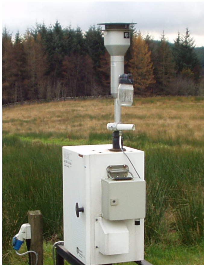
Image 4. The Partisol 2000 sampler at the Network monitoring site at Eskdalemuir. The grey box attached to the side of the sampler contains the mercury vapour sampling equipment.
