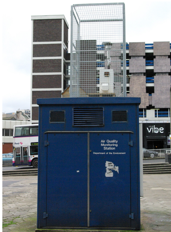
Image 3. The Network monitoring site at Sheffield Centre AURN where mercury vapour monitoring equipment was installed in June 2009.
