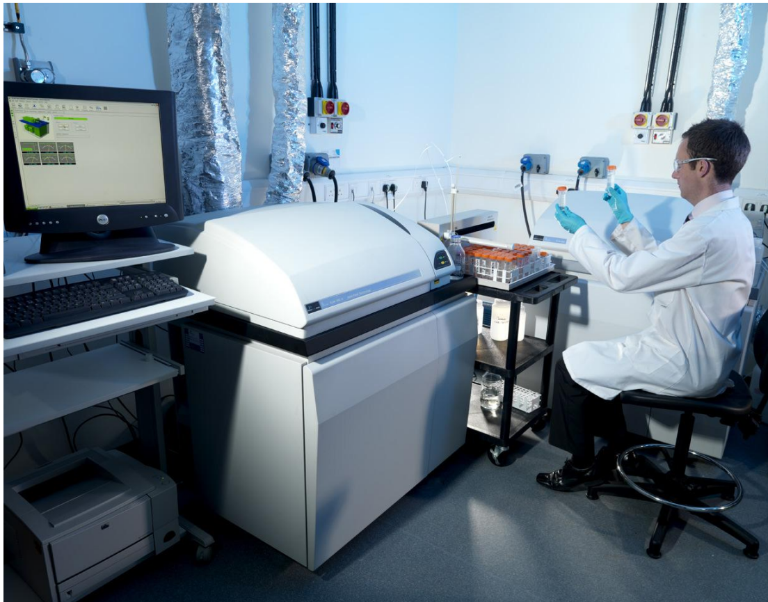
Image 3: One of two dedicated ICP-MS instruments comprising the UK ambient metals analysis facility at NPL.
