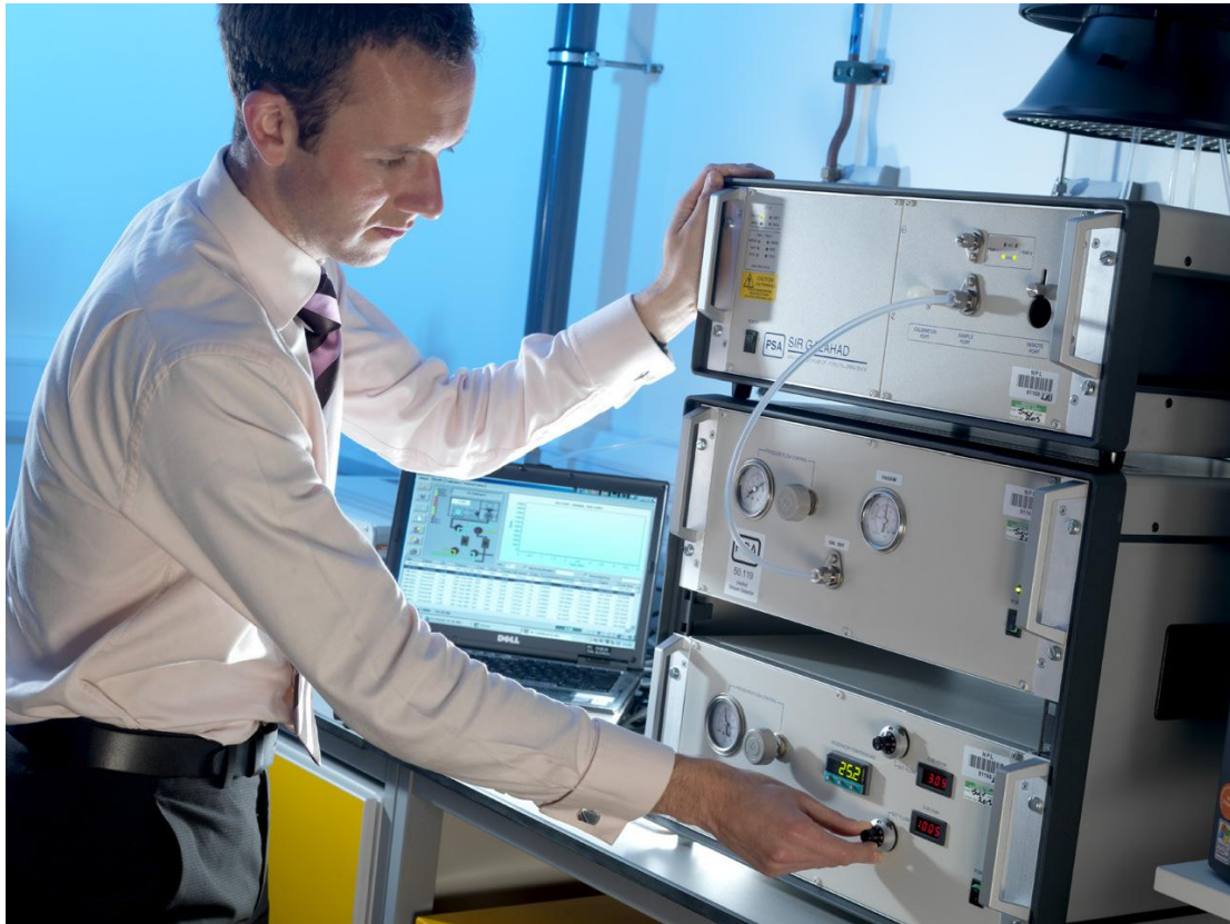
Image 4: One of two thermal desorption-atomic fluorescence analysers comprising the UK total gaseous mercury analysis facility at NPL
