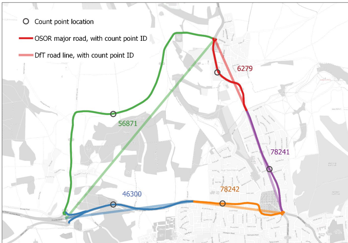
Figure 11-3 Traffic flows are assigned to the road network (Ordnance Survey Open Roads) by selecting OSOR sections that fall between the start and end points of traffic census count point coverage (DfT road line)
