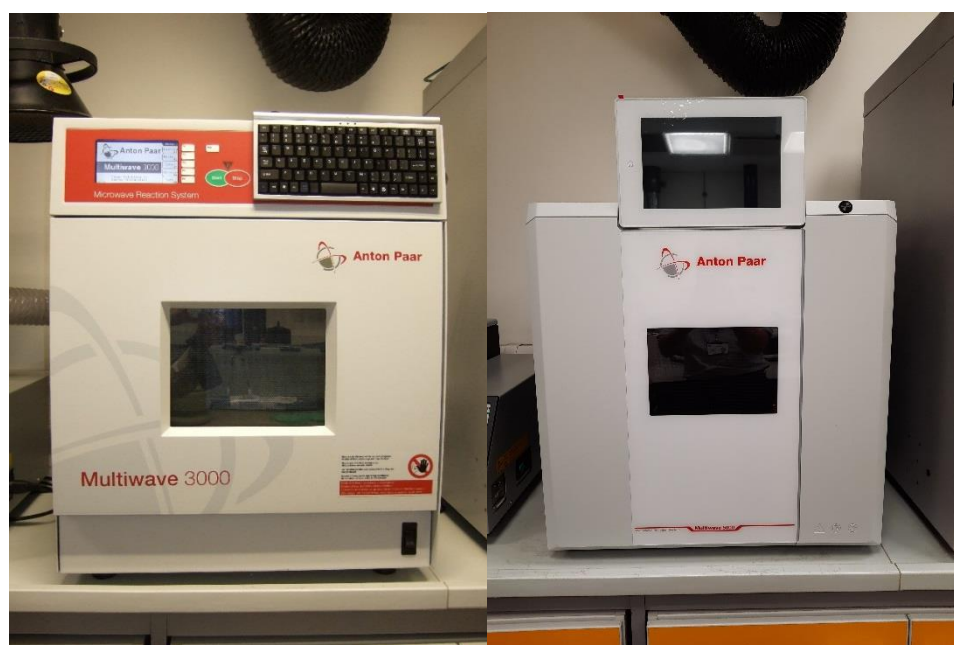
Image 2 Anton Paar Multiwave 3000 (left) and Multiwave 5000 (right) microwaved used for acid digestion of the sampled filters.
