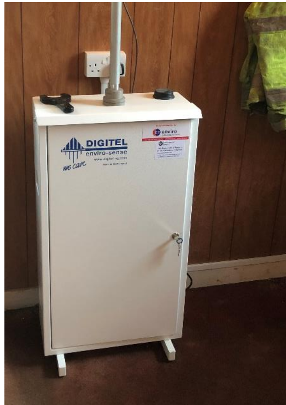
Image 1 The Digital DPA14 sampler at the network monitoring site at Swansea Coedgwilym.
