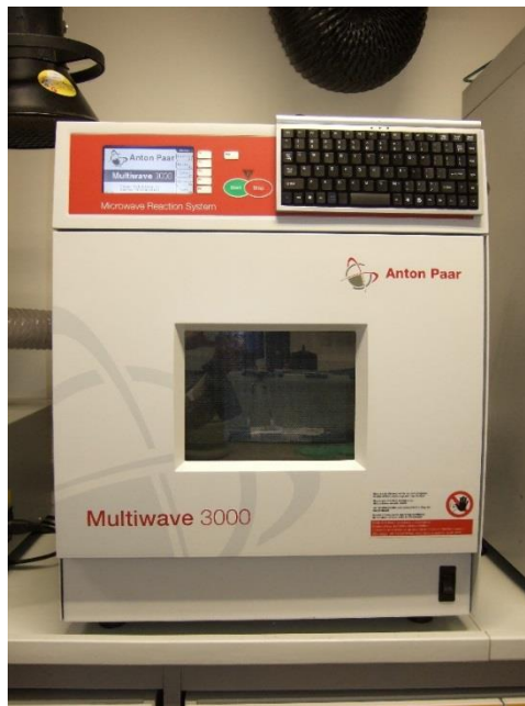
Image 2 Anton Paar Multiwave 3000 microwave used for acid digestion of the sampled filters.
