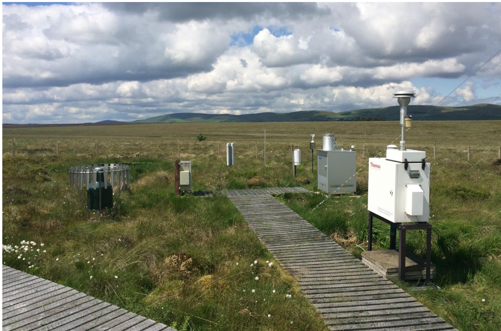
Image 4 Partisol sampler (foreground) at Auchencorth Moss. Picture courtesy of Matt Jones (UKCEH).
