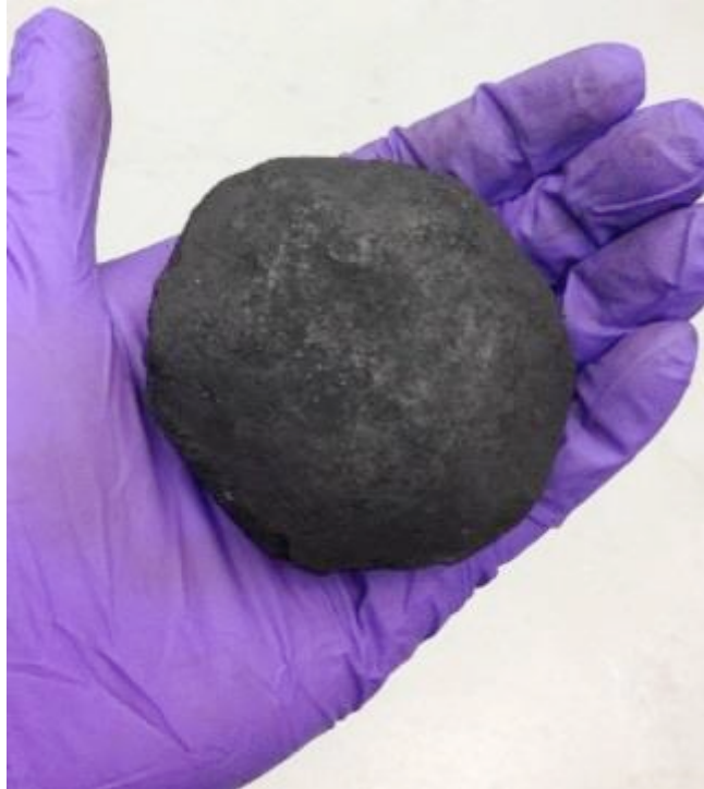
Figure 8: Example of biocoal 50:50 biomass and coal blend briquette [CPL]
