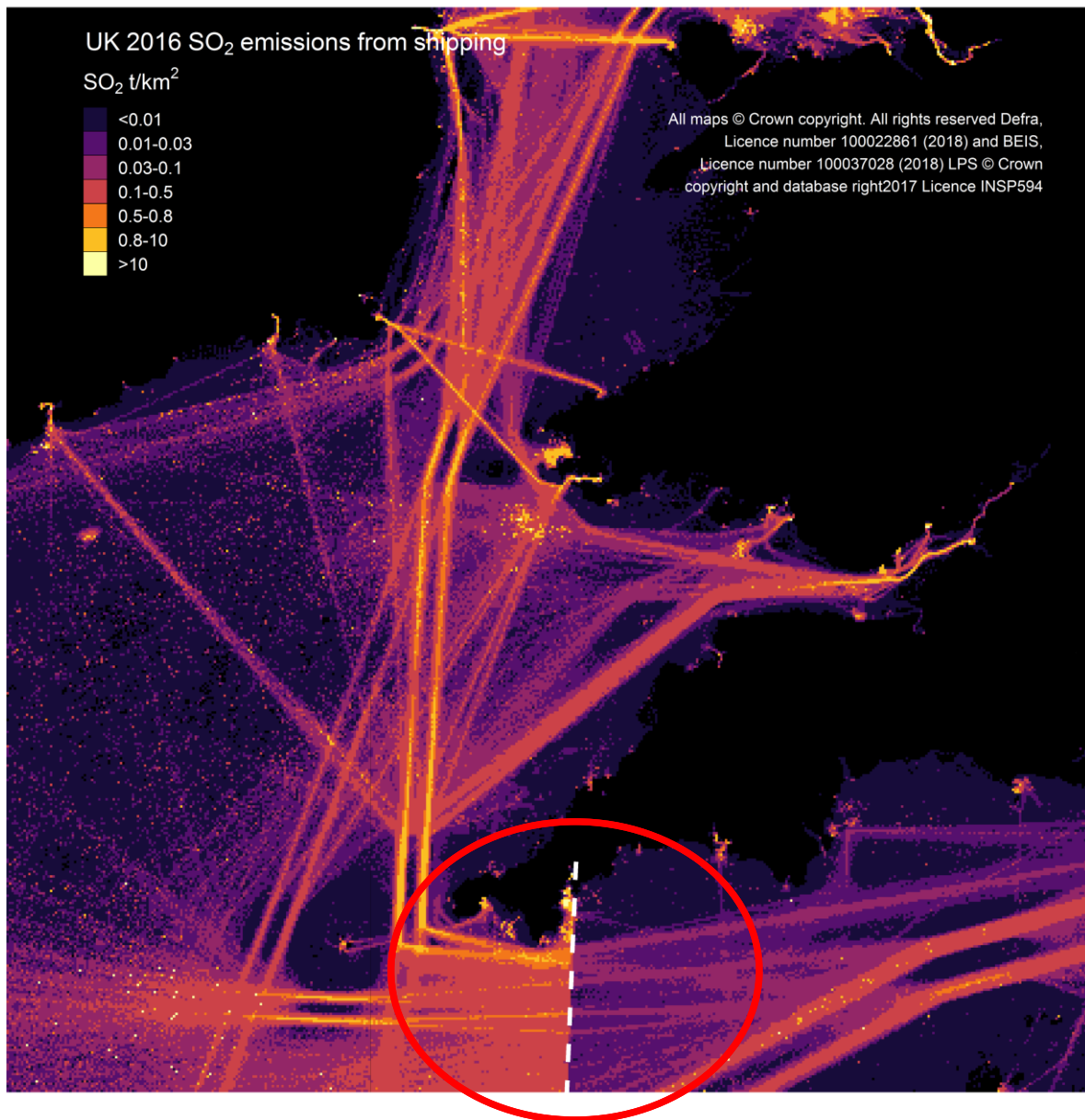
Figure 11-8 SO 2 emissions from all shipping around the south-west of the British Isles. The SECA (Sulphur Emission Control Area) to the east of the dotted white line (bottom centre) can be seen as a reduction in emissions
