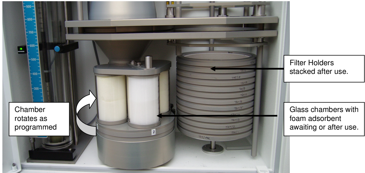
Figure 4: Picture of a Foam Adsorbent Auto Changer for the Digitel DHA-80 Sampler
