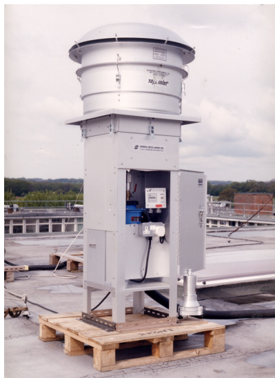
Figure 2: Andersen GPS-1 Sampler
